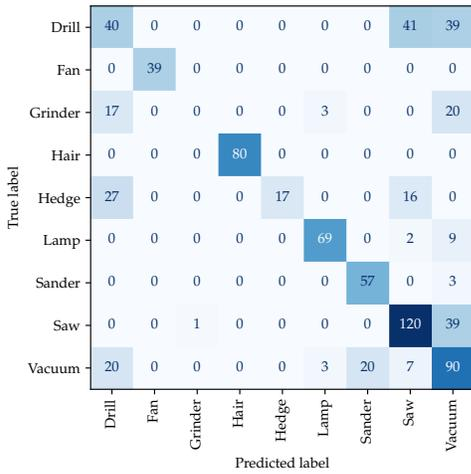
Fig. 4. Confusion matrix of leave-one-house-out test split result on COOLL dataset. Cross validation results have been aggregated.
