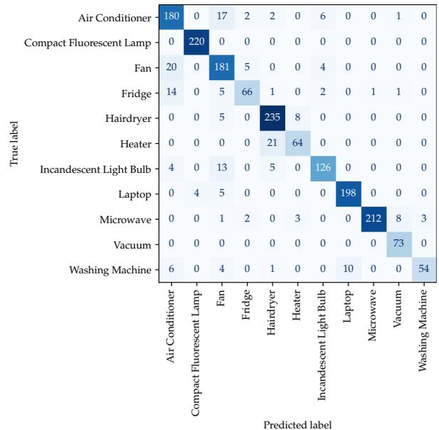
Fig. 6. Confusion matrix of leave-one-house-out test split result on PLAID dataset. Cross validation results have been aggregated.
