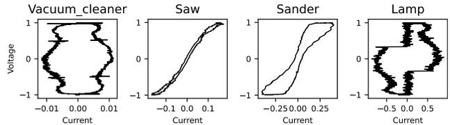
Fig. 1. Standard V-I trajectory plots where current and voltage are plotted against each other. Examples are taken from the COOLL dataset. The data are scaled to range  $-1$  to  $+1$ .
