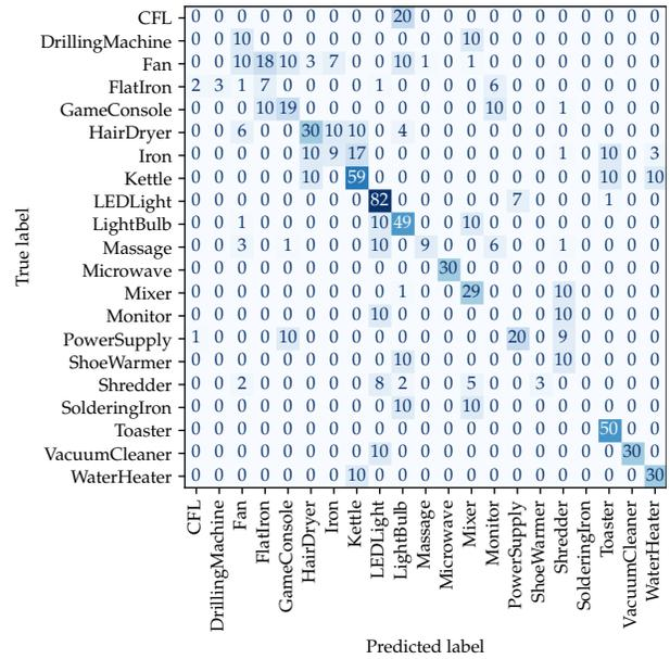
Fig. 5. Confusion matrix of leave-one-house-out test split result on WHITEDv1.1 dataset. Cross validation results have been aggregated.
