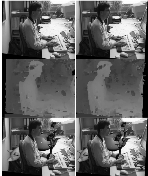
Figure 7. roffice image pair, taken by a hand-held camera. Top: rectified images. Middle: Disparity maps for parameters roff1 . Bottom: Augmented scene
